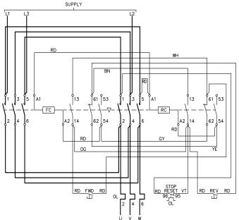
SEPARATE NO-VOLT SUPPLY: REMOVE LINK BETWEEN 1 ON RC & 96 ON OL AND 5 ON RC & A1 ON RC. CONNECT SEPARATE SUPPLY TO 96 ON OL & A1 ON RC.
