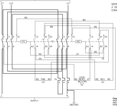
REMOVE WHITE LINK (13 ON FC-61 ON RC) REMOVE BROWN LINK (13 ON RC-61 ON FC)
