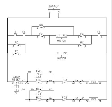
SEPERATE NO-VOLT SUPPLY: REMOVE LINK BETWEEN 2 ON FC & 96 ON OL AND 6 ON OL & A1 ON RC. CONNECT SEPERATE SUPPLY TO 96 ON OL & A1 ON RC.
