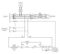
FOR LINE & NEUTRAL CONTROL, REMOVE LINK BETWEEN A1 & 5 ON C AND WIRE AS SHOWN DOTTED.
